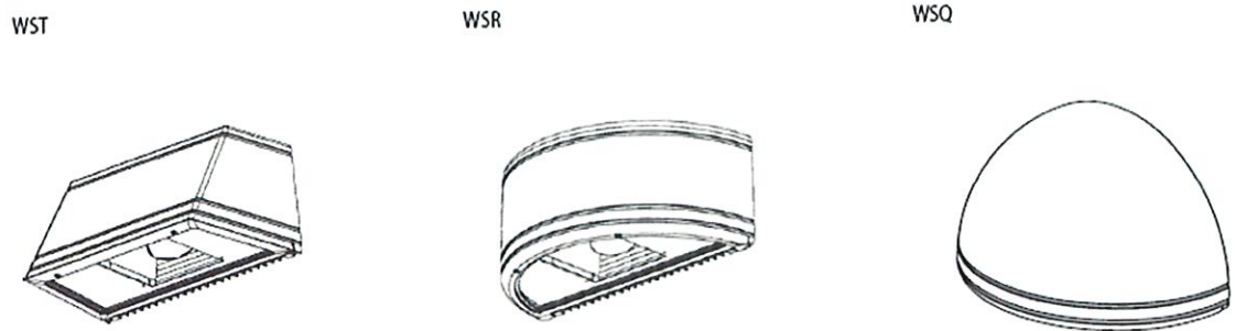
Figure L: Samples of acceptable wall packs.
